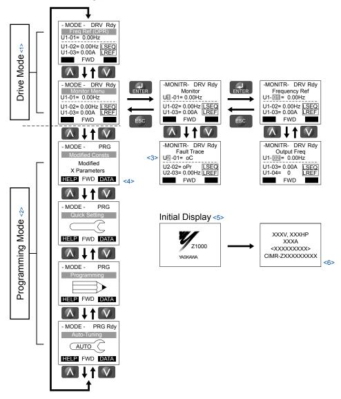
Figure i.14 HOA Keypad Menu and Screen Structure
