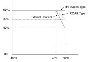
Figure i.18 Ambient Temperature and Installation Method Derating
