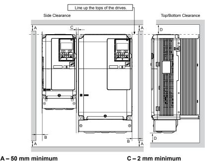
Figure i.3 Space Between Drives (Side-by-Side Mounting)
