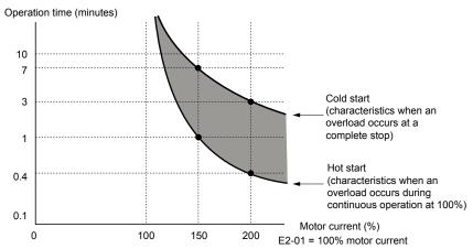
Figure i.17 Motor Overload Protection Time
