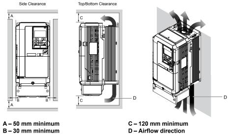
Figure i.2 Correct Installation Spacing
