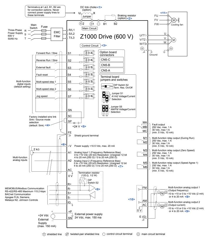
Figure i.5 Drive Standard Connection Diagram
