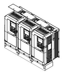
Figure i.4 IP20/UL Type 1 Side-by-Side Mounting in Enclosure
