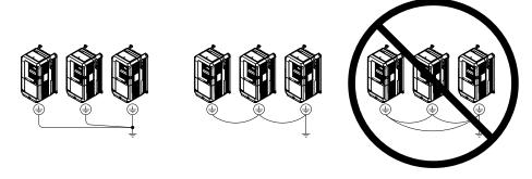
Figure i.6 Multiple Drive Wiring
