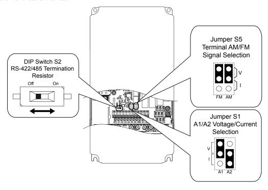
Figure i.12 Locations of Jumpers and Switches on the Terminal Board
