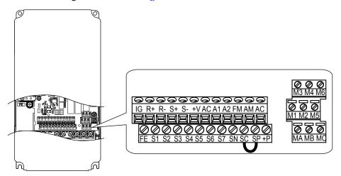
Figure i.7 Control Circuit Terminal Arrangement
