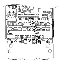
Figure i.10 Terminal Board Location Inside the Drive
